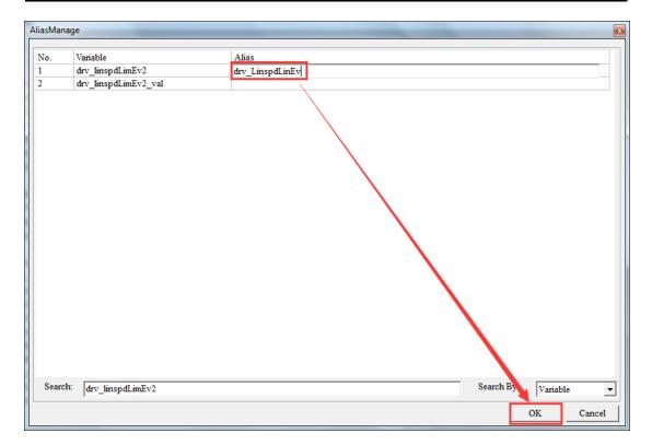
3) Alias of 'drv\_linspdLimEv2' is replace by 'drv\_linspdLimEv'.
