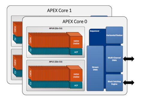
The APEX core provides flexible configuration at runtime. By default, APEX is configured as a single APU with 64-CU. When using the APEX Core Framework library, you can change the configuration at runtime and have two separate APUs, each with 32 CUs. For information on how to use APEX to program, please download <u>Vision SDK Software</u> and refer to the documentation, or you can use the S32 Design Studio for Vision IDE.
